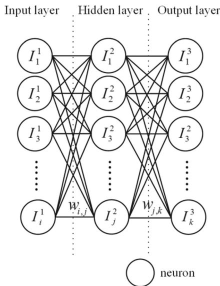
**Fig. 2** The structure of a three-layer ANN (modified from Basheer and Hajmeer (2000))
