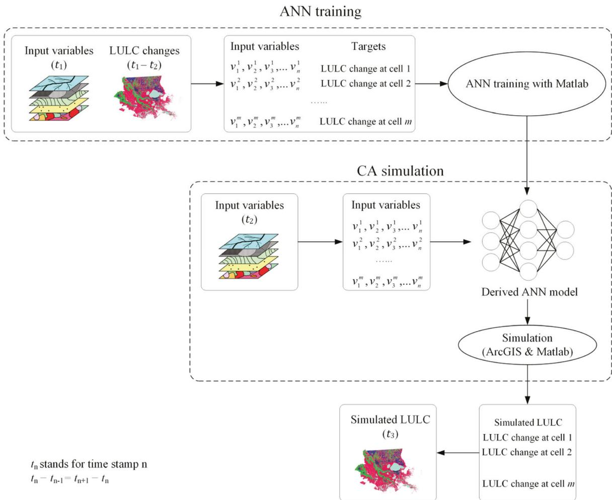
**Fig. 4** The workflow of the training and simulation processes
