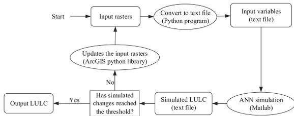
**Fig. 5** The interaction between ArcGIS® and Matlab® in the simulation
